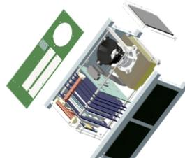
Figure 1 : QlevEr Sat Nanosatellite
